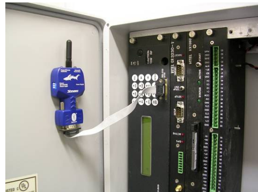
Stevens Bluetooth RS232/RS485 adapter attached to a datalogger in an industrial environment.
