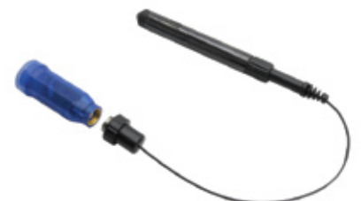
Diver Mate hand-held data download and storage drive
