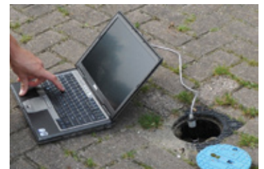
USB Interface Cable attached to Diver Data Cable from laptop computer
