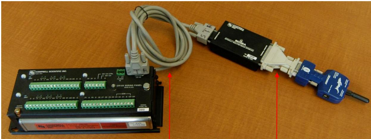
9 pin male to 9 pin female straight-through serial cable
