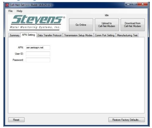
In this tab, you can set the APN (Access Point Name) User ID, and Password for the Cellular network associated with the installed SIM (subscriber identity module) card. Many times a User ID and Password is not needed. In this case, leave these fields blank.
