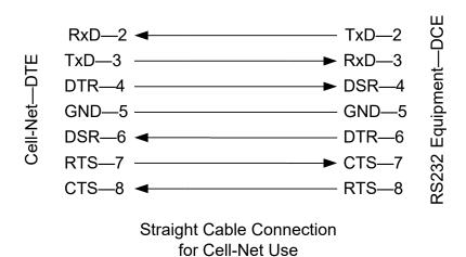
Stevens Cell-Net can be connected to a DCE such as a data logger or any other RS232 device using a straightthrough cable.
