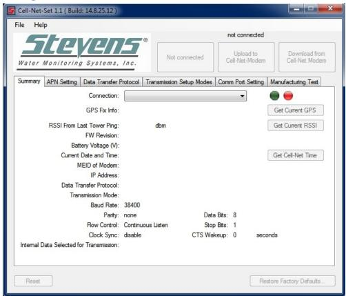
When the software is first opened, the "Go Online/Go Offline" Button (see section 4) will say that it is not connected near the top. In the summery tab, click the down arrow in the connection box. If the modem is connected through the USB, the MEID or IMEI of the connected modem will appear. In this example, the IMEI number is 354660047225845, but will be different for every modem.
