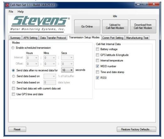
In the Transmission Setup Modes Tab, the user can select and control the data transmission criteria.
