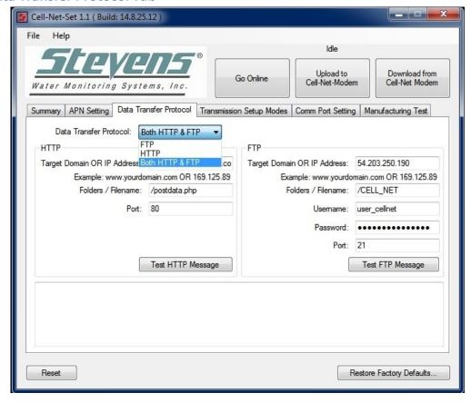
In the data transfer protocol tab, the destination to either an FTP, HTTP or Both HTTP & FTP can be configured.
