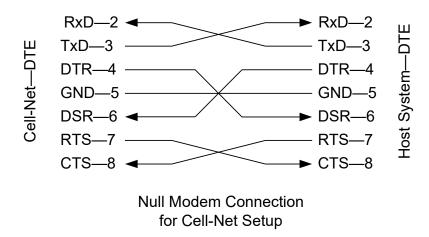
Stevens Cell-Net is a DTE, Use this pinout configuration when connecting the serial comm port to another DTE such as a computer. Note that you will need a null modem cable or a null modem with a straight through cable to connect to a computer through the serial port.
