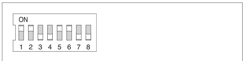
Fig. 20: Factory setting of the operating parameters.
