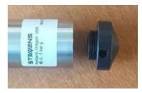
The Smart PT ships with an engineered resin cap designed to protect the ceramic membrane. It's important to remove the cap if the Smart PT is expected to freeze. If the cap isn't removed, expanding ice trapped under the cap will damage the ceramic membrane.
