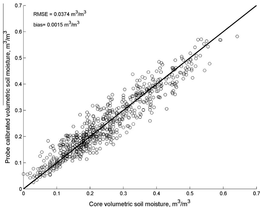
Fig. 6. Comparison of volumetric soil water content measured from the gravimetric core samples and the calculated volumetric soil water content, with individual field equations applied to data from the appropriate field. The solid line is the 1:1 line.
