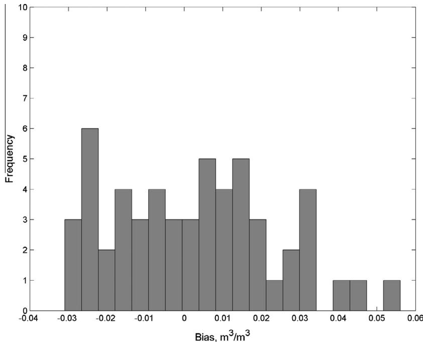
Fig. 4. Histogram of the bias values for each field using the general Eq. (8) for the calibration.
