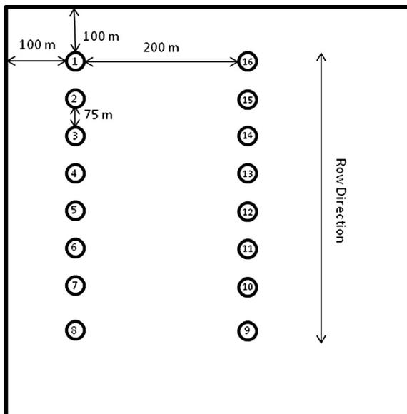
Fig. 2. Diagram of the manual soil moisture sampling transects. Sampling would begin at point 1 and progress in numerical order until point 16. The diagram is not drawn to scale.
