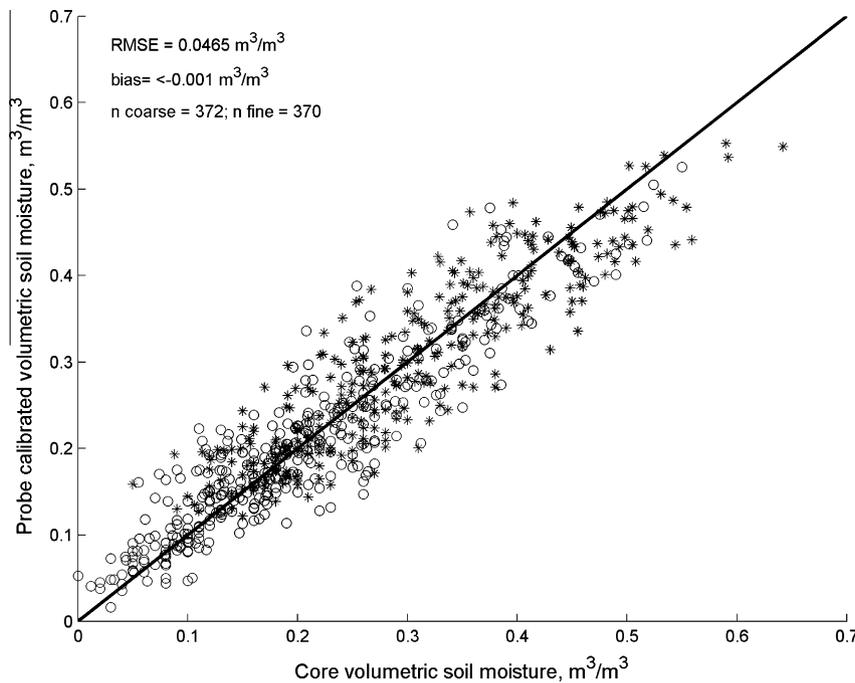
**Fig. 5.** Comparisons of volumetric soil water content measured from the gravimetric core samples and the calculated volumetric soil water content using (9) and (10). The circles represent the coarse textured soils, and the stars those with clay content >40%. The number of points used in establishing the model for the coarse and fine textured soils were 371 and 370, respectively. The solid line is the 1:1 line.
