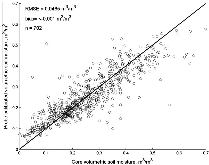
**Fig. 3.** Comparison of volumetric soil water content measured from the gravimetric core samples and the calculated volumetric water content using (6). The number of samples used in the establishment of (6) was 702. The solid line is the 1:1 line.
