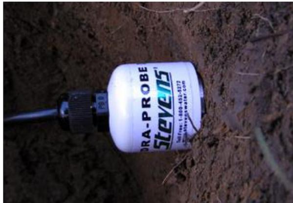
**Figure 2.6** HydraProbe Installed in undisturbed soil.
