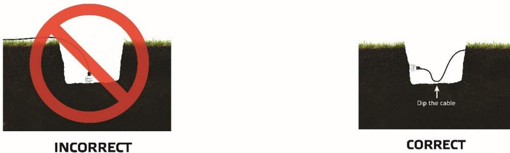
**Figure 2.7** Horizontal placement sensor and dipping the cable is recommended
