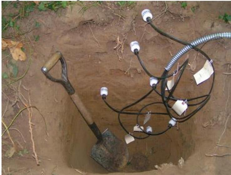
**Figure 2.3 Six HydraProbes installed into 6 distinct soil horizons.**
