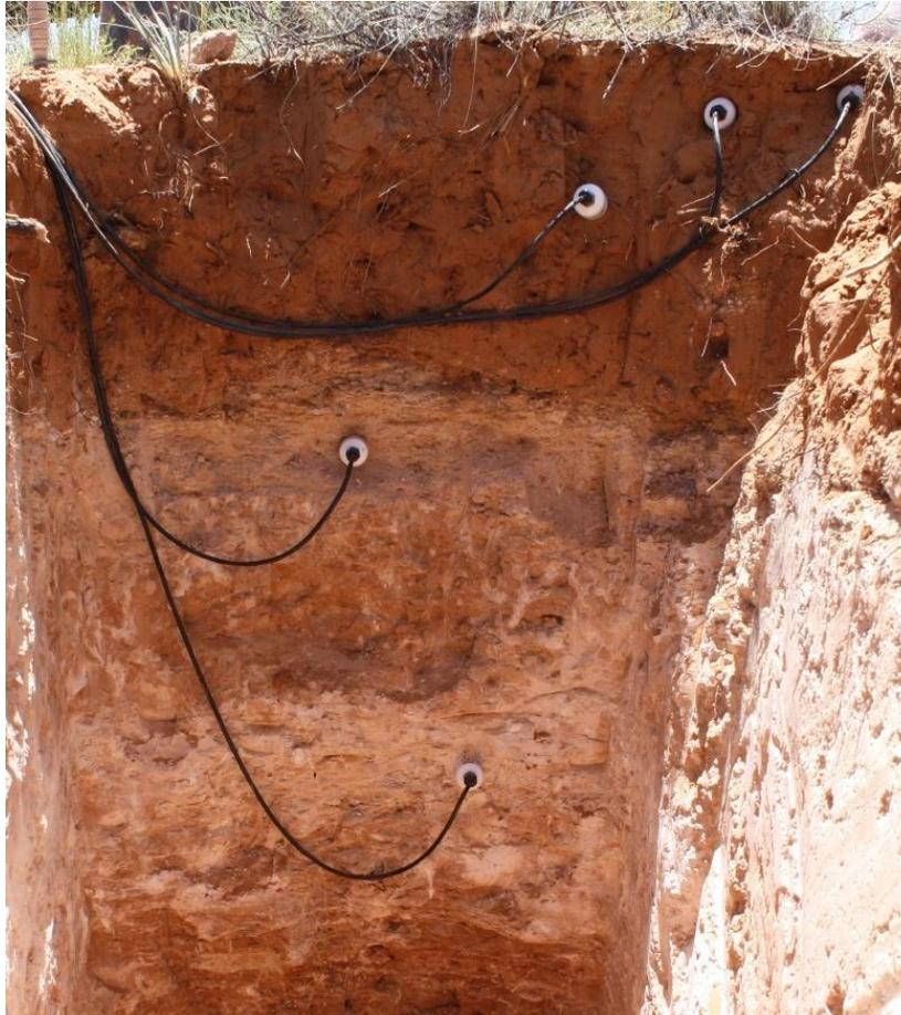
HydraProbe installation at a typical USDA NRCS SNOTEL Site.
