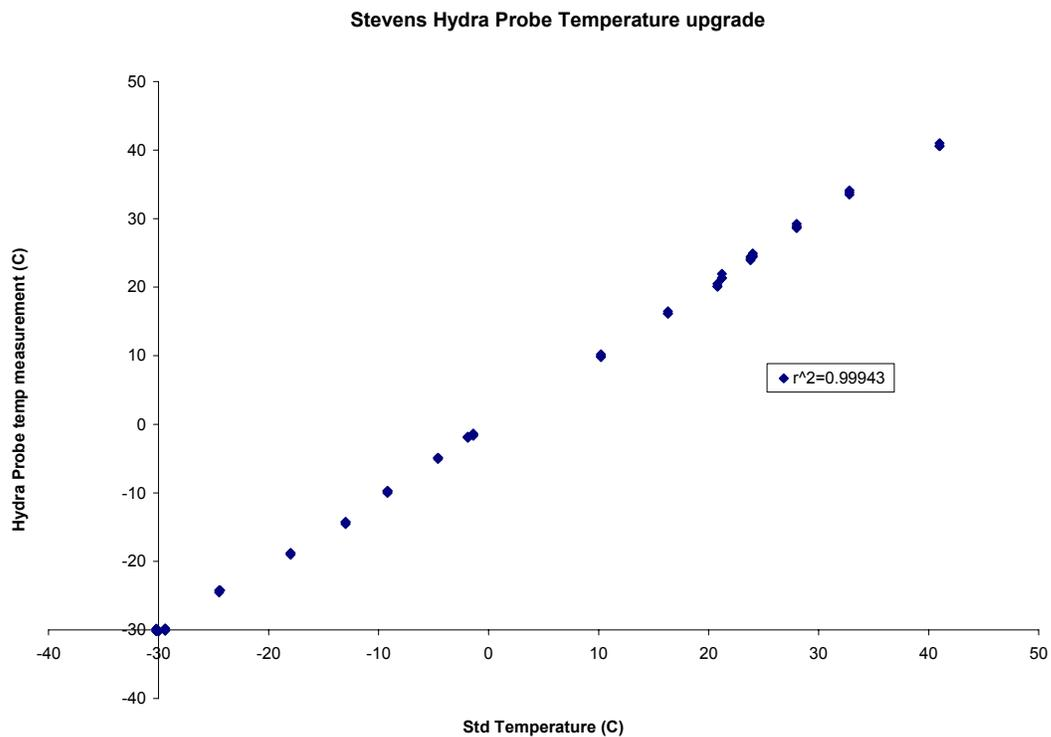
**Figure 1. Plot of Hydra Probe Proto Type vs. a Standard thermistor.**
